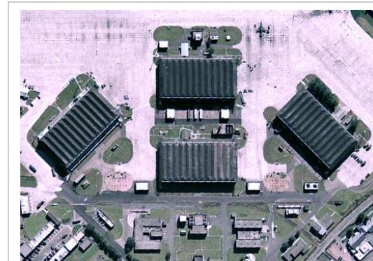
Some specialist technical equipment needs to be sited at a distance from domestic areas of the airfield. Here, two engine **de-tuners** can be seen on a hardstanding; these are used to test jet engines before re-fitting to aircraft.
